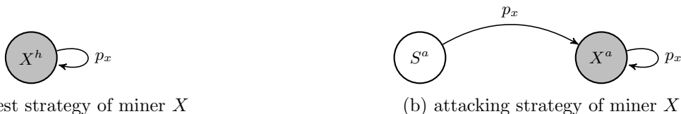
Figure 7: The honest strategy (cf. Figure 7a) and deviation from the honest strategy (cf. Figure 7b) modeled with discrete Markov chains. All states with a nonzero payout for miner X are highlighted in gray. We transition between states with every block. Note that for all remaining probabilities, the Markov process enters an absorbing state and X ’s consecutive turns as a proposer finish.
